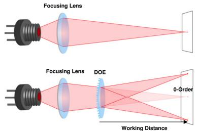
Laser diodes are the most common light source to be used with diffractive optical elements, but other laser light sources may also be used.
